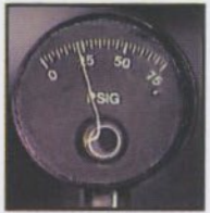
RESERVOIR AIR PRESSURE GAGE
