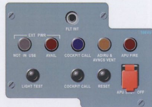
EXTERNAL POWER PANEL (108VU)
